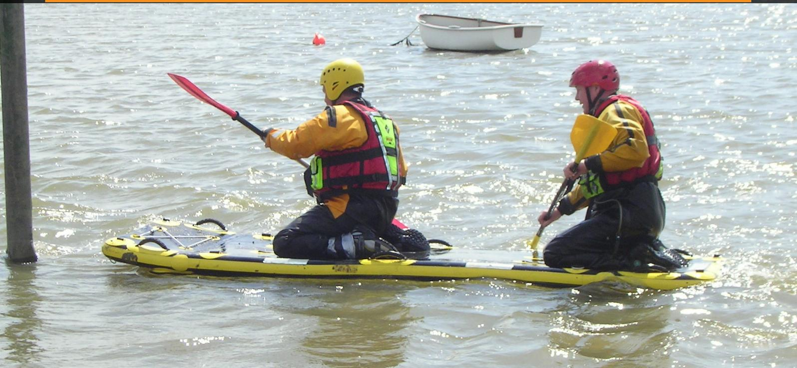
The RP3 is an inflatable platform for the recovery of casualties primarily in shallow water, mud, ice and swamp environments. The RP3 provides a very stable rescue platform due to its catamaran style sponsons. Where necessary the platform can be operated behind a jet ski or with fast rescue craft, and is also easily paddled or line transferred.
