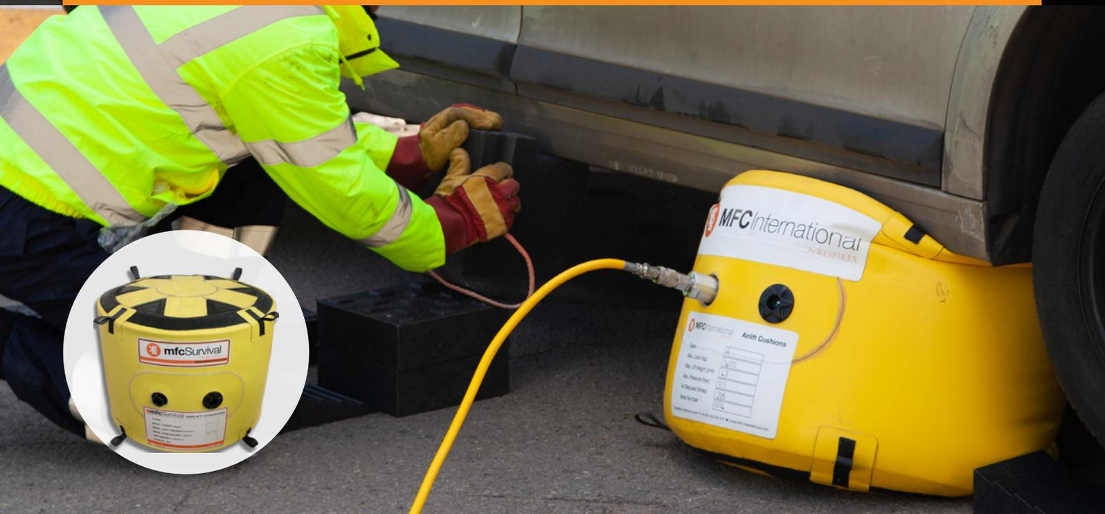
MFC International offer a comprehensive range of low pressure 0.5 bar (7 psi) lifting bags, designed primarily for the recovery of vehicles.
