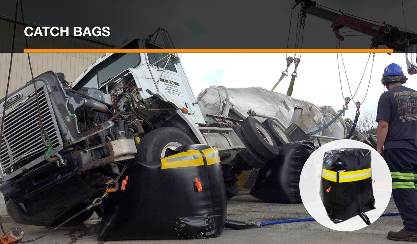
MFC International Catch Bags are designed to be used in conjunction with our low-pressure high-lift air bags during the up-righting of vehicles or trailers.
