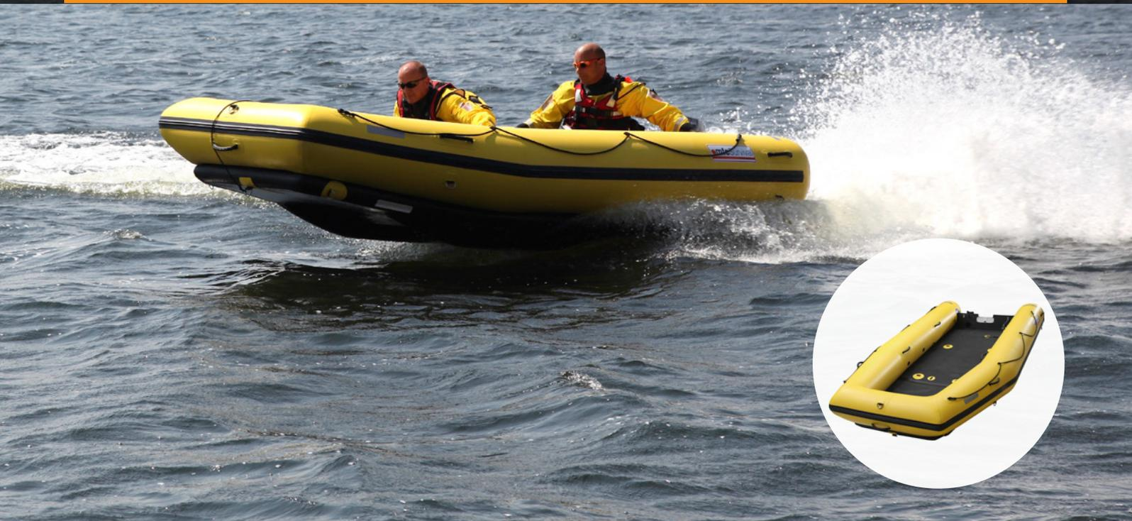
The RC4000 Rescue Craft from MFC International is designed to meet the performance criteria of a conventional Inflatable flood rescue boat, while providing the shallow draft and ease of transportation of a rescue sled. The inflatable four-meter design incorporates twin keels with the rigid inflatable floor.
