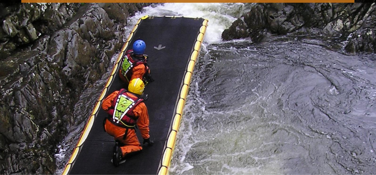
The Airtrack is an inflatable rescue path used by the majority of the rescue services for accessing casualties during rescue on water, mud, ice and unstable terrain.
