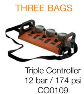
MFC's 12 bar aluminium control units are robust and durable with an impact resistant design. The controller features a pressure sensitive 'deadman' control joystick and a pressure gauge with protective rubber surround for each controlled outlet. The body is made of aluminium with plastic protective handles at either end and models are available for control of one, two or three bags. The controller is supplied as standard with a female type 26 inlet coupling and Type 25 female couplings.
