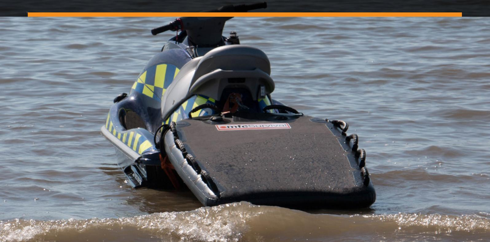
The Jet Ski Rescue Board is an inflatable board that is designed to be attached to the back of a jet ski to aid rapid response and rescue of casualties. It is attached by three towing and control 'D' rings located at the front of the inflatable board.
