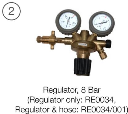
Regulators are designed to be used with an air cylinder to reduce the amount of pressure which is leaving the cylinder and entering the inflatable product. The regulator contains an on/off valve which stops the air flowing through the hose.
