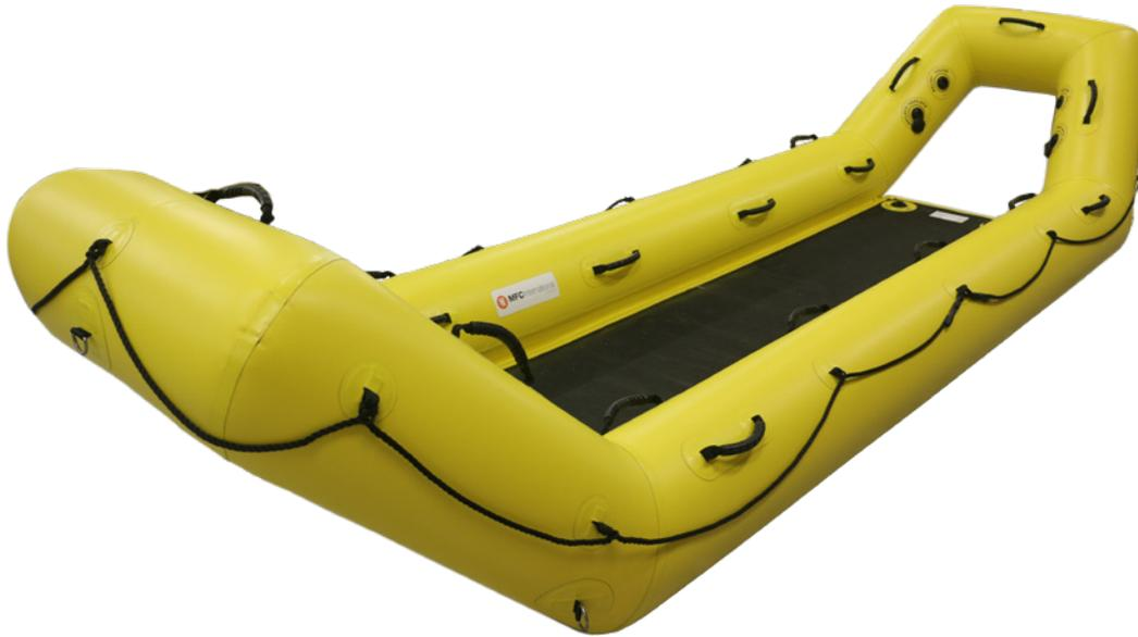
The RSW Rescue Sled is fitted with extended tubes which provide its unique design. Based on the design of the standard Rescue Sled, it provides options for rescuing casualties from difficult situations such as weirs.
