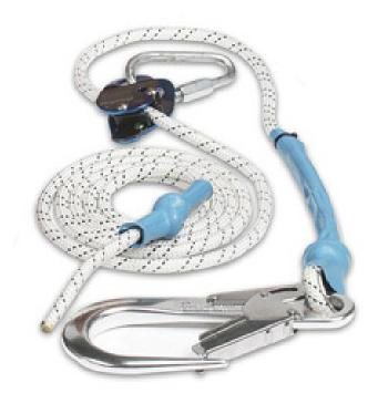
Our securing lanyard consists of 10.5mm diameter nylon static rope, rocker rope grab and an aluminium snap hook (colours may vary). The securing lanyard has no specified break load on account of the use of knots in the construction, which can weaken the rope MBL by c.50%.
