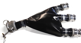
Distributor, 3-Way [Camlock 1½" Skt x1, Plg x3] (SP0157)
