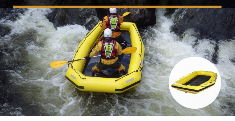
Fully inflatable, the Evacuation Raft is lightweight and portable. It is easy to manoeuvre, and can be paddled or pulled by hand. The Evacuation Raft has a flat bottom, making it exceptionally stable and suitable for use in very shallow water from 50mm in depth. The Evacuation Raft is ideal in flood rescue situations.
