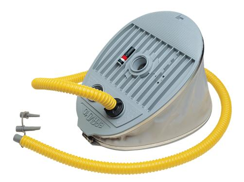
The Bravo 10 foot pump utilises an innovative design to make inflating and deflating a tube as effortless as possible. It has two chambers, one 5 litre (high volume, low pressure) which inflates to 2.1 psi and one 1.6 litre (low volume, high pressure) which inflates to 4.4 psi.
