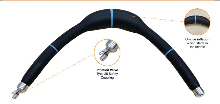
MFC T90 Packers are constructed using unique flexible rubber materials making them lightweight, flexible to manoeuvre and can inflate to repair pipes with 45°, 60° and 90° corners. T90 Packers are easy to operate and are specifically designed to simplify the process of inserting/removing a packer through a tricky pipe system.
